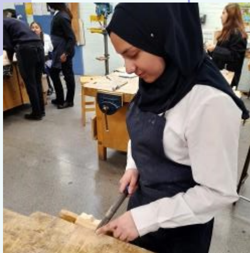
Amani using a range of files to finish the edges of the timber
